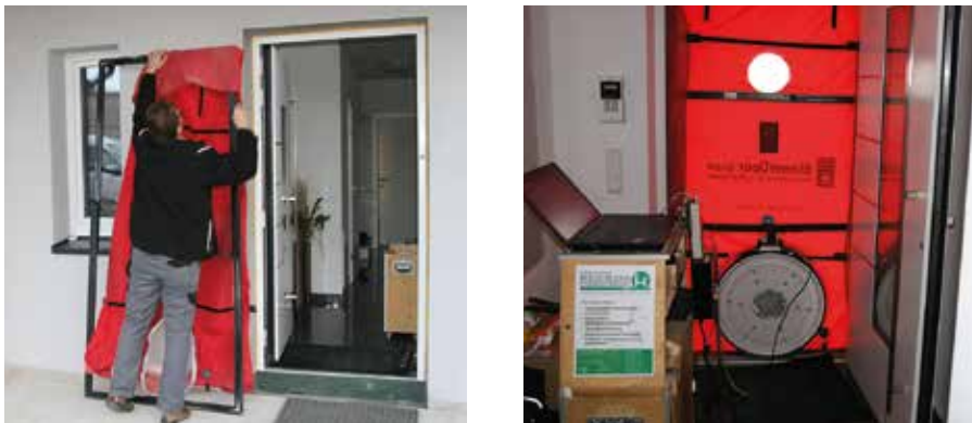
Fig. 10 | Measurement equipment for the blower door test. © vōz
